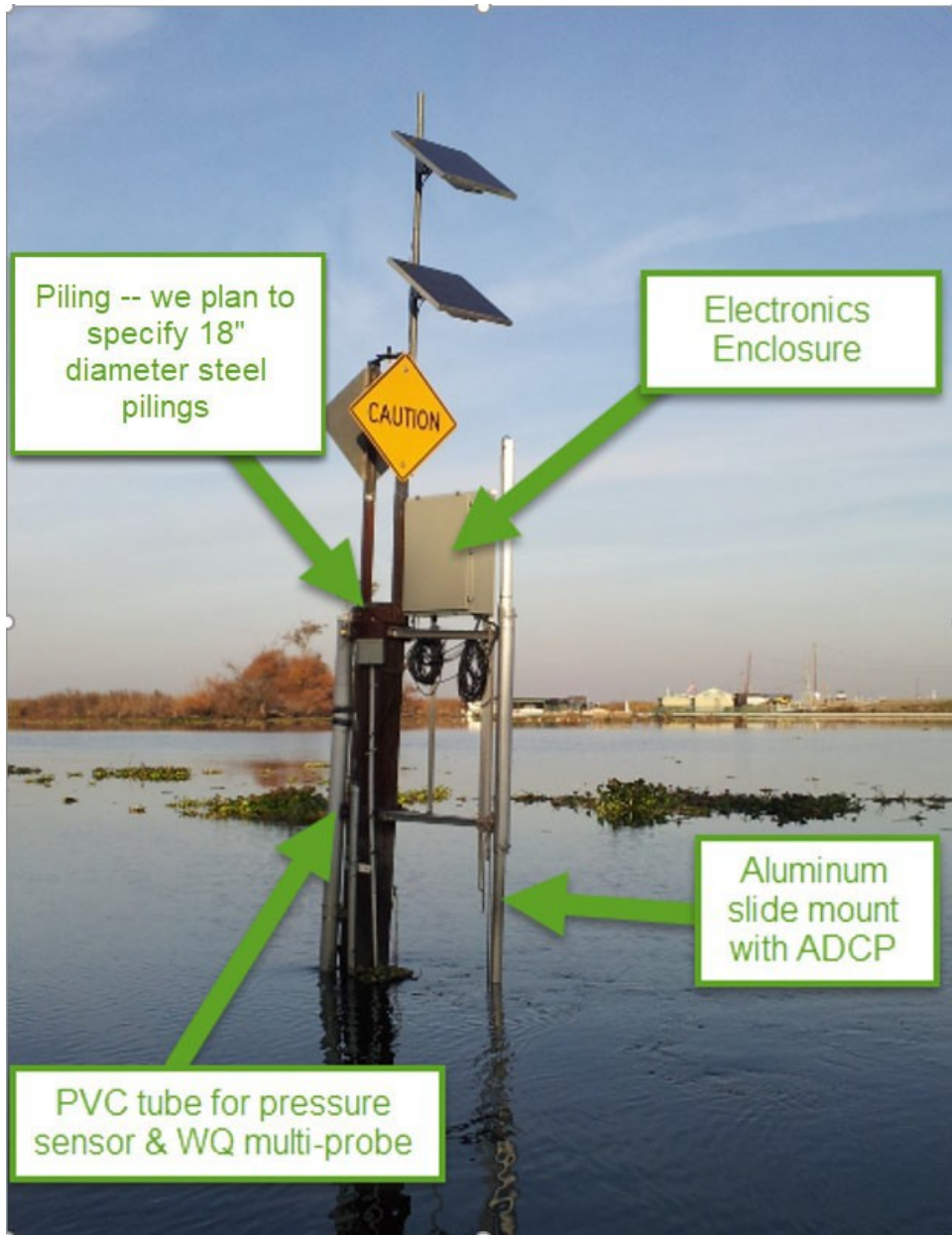
Figure 1: Standard configuration of a Delta Flow and Water Quality Monitoring Station
